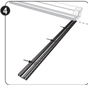
**4** The fixed profile of the coupling side guiding channel fastened centrally every 250 mm via the removable profile of the curtain wall to the clamping strip.
